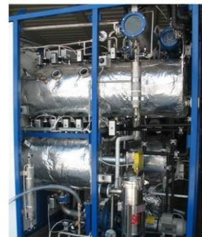
Each section has an inspection window, a level sensor and a series of automatic valves that open/close after completion of the various steps as defined in the program for the selected cleaning process. The third and fourth sections are heated by electrical heaters directly immersed in the solvent.
