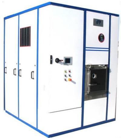
The single cleaning chamber is utilized for all stages of the cleanliness cycle including spray cleaning, immersion cleaning, optional ultrasonic cleaning, rinsing, drying and optional rust inhibitor application.
