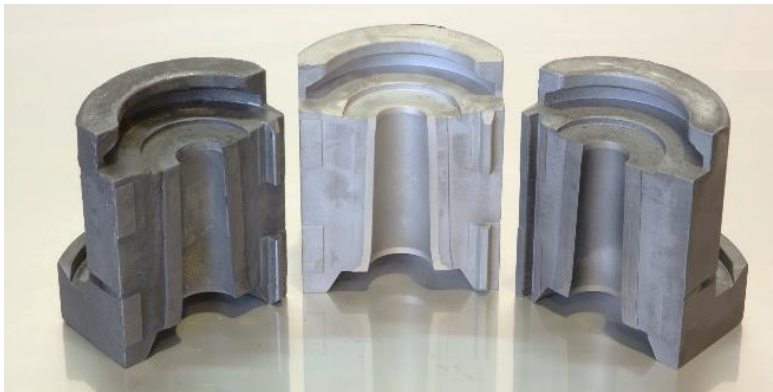
Glass moulds before washing (left), cleaned with ultrasound (middle) and sand-blasted (on the right).
